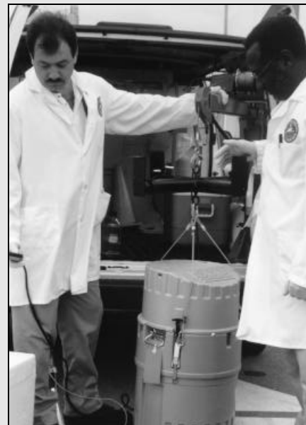
Picture 4. The fixed crane makes it easier for one or two of the City of Hollywood Pretreatment Compliance Inspectors to safely raise and lower their composite samplers.
