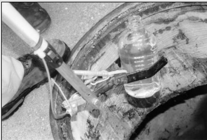
Picture 3. A close-up of the sampling pole with articulating head.
