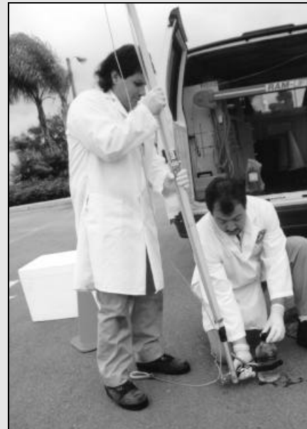
Picture 2. City of Hollywood Pretreatment Compliance Inspectors demonstrate the use of their home-made sampling pole.
